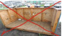
A typical job-made box consists of a wooden platform with three walls. In this example, the job-made box was attached to a powered industrial truck (PIT) using a strap looped around the center of the wood beams that make up the longest wall and a galvanized hook. A worker was injured when the hook's safety latch failed and the platform fell to the ground.
